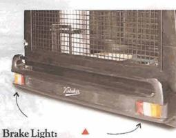
While towing the compressor on highway, it is mandatory for the vehicle to have proper break lights. This feature is provided in this compressor through a port, which can be connected to the break lights of the towing vehicle.
