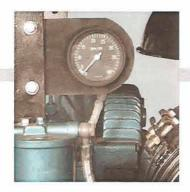
Engine RPM Meter:
